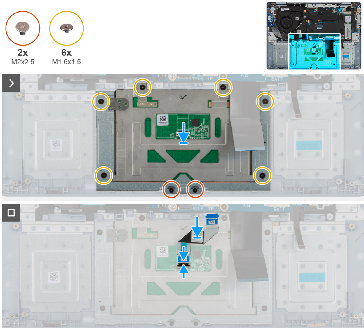
Figure 39. Installing the touchpad
